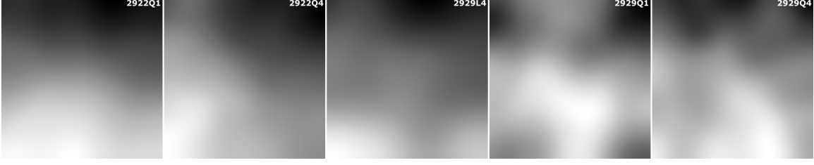
Figure 2: Estimated intensity inhomogeneity (bias) field for each of the five data sets.
